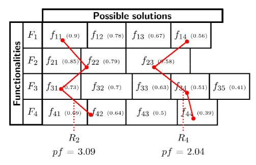
Fig. 6. Exemplary preference factors of particular elements of a morphological table (values in brackets) and selected solutions of a diagnostic system, pf – preference factor
