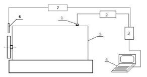
Fig. 1. Diagram of the measuring system: 1 – vibration acceleration sensor, 2 – preamplifier, 3 – terminal connection, 4 – portable computer, 5 – investigated internal combustion engine, 6 – location of the crankshaft sensor, 7 – power pack
