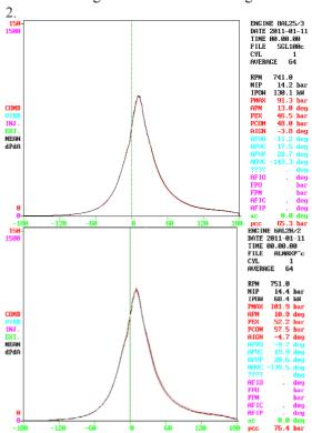
Fig. 2. Chosen engine cylinder pressure diagrams with other parameters for close to rated power load – main engine 8AL25/30 type (up), - auxiliary engine 6AL20/24 type (down)
