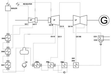
Fig. 1. Functional scheme of a power block [2]. (EX: steam extraction port; XW: high pressure heater; XN: low pressure heater; CO: condenser; PZ: main pump)
