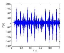
Fig. 10. Signal from model for incorrect work due to misalignment of the gears, with high loading and rotational speed 800 RPM
