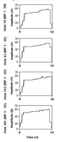
Figure 8: Raw spindle motor current signals for the time period of specific drillings
