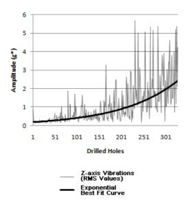
Figure 9: RMS values of the obtained vibrations and the related best fit curve  $(*g=9.81 \text{ m/s}^2)$
