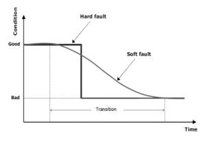
Figure 1: Hard and soft faults, Courtesy of [2]
