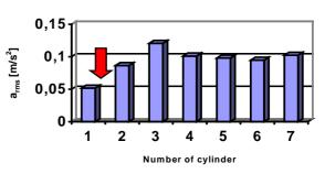
Fig. 9. Root-men-square values of accelerations vibrations signal by the sensor fastened on the cylinder head cover screws for 1–7 cylinders of 7L16/24 engine: ↓ – failed of piston-cylinder group after restart the engine
