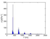
Fig. 9. PSD for signal from model for correct work of the gears, with high loading and rotational speed 800 RPM
