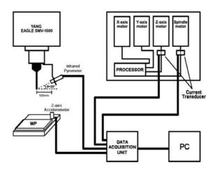
Figure 3: The experimental set-up
