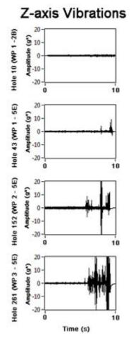
Figure 6: Raw Z-axis vibration signals for the time period of specific drillings ( $*g=9.81 \text{ m/s}^2$ )
