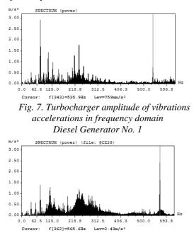
Fig. 8. Turbocharger amplitude of vibrations accelerations in frequency domain Diesel Generator No. 2
