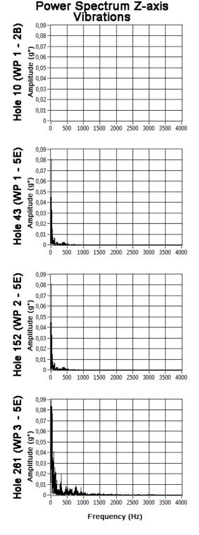
Figure 13: FFT analysis of the obtained vibration signals (\*g=9.81 m/s<sup>2</sup>)
