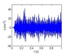
Fig. 4. Signal measured in the experiment for incorrect work due to misalignment of the gears, with high loading and rotational speed 800 RPM
