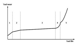
Figure 2: Tool wear evolution: (1) initial wear, (2) slight wear, (3) moderate wear, (4) severe wear and (5) worn-out
