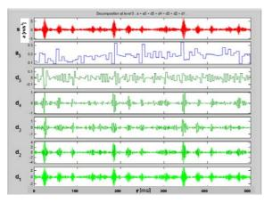
Fig. 7. Wavelet analysis of the accelerations vibration signal: s – registered basic signal,  $a_5$  – low-pas filter,  $d_4$ – $d_1$  – high-pas filter
